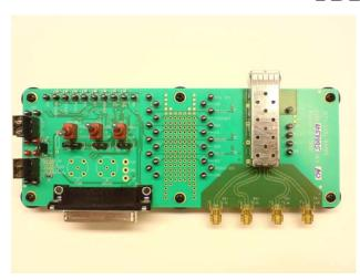
Finisar's FDB-1027 Evaluation Board is the perfect vehicle for testing and evaluating SFP/SFP+ optical transceivers.
